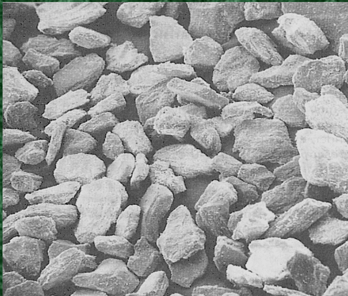
Powder particles of plaster of Paris
