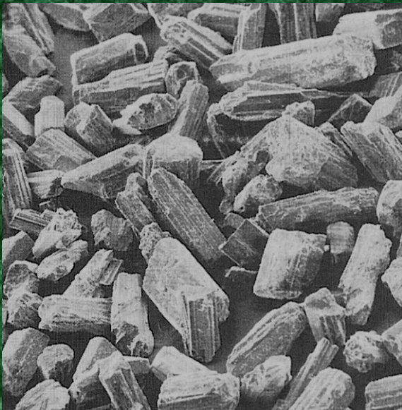
Powder particles of dental stone
