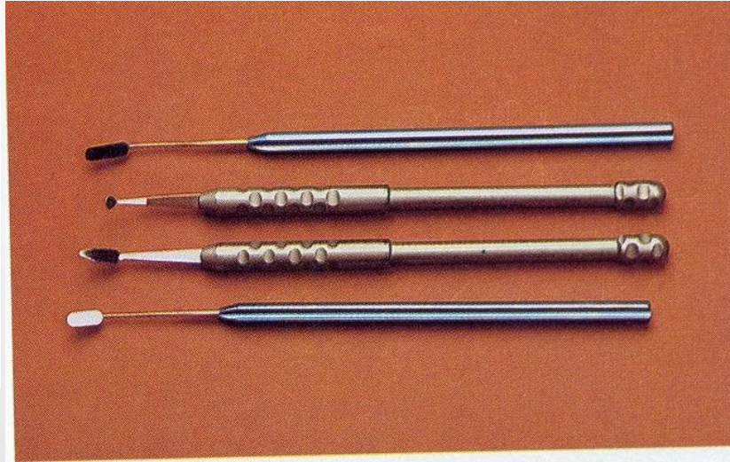
Fig. 4-10 Micromirrors with sapphire surfaces ( center ) and stainless steel surfaces ( top and bottom with blue handles ).
