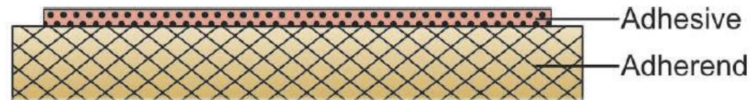
Fig. 16.1: Adhesive and the adherend
