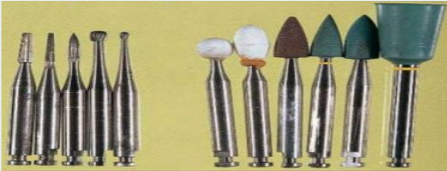
Fig. From the left: five plain-cut plain steel finishing burs, two mounted stones, three mounted abrasive rubber points from coarse to fine, and a mounted abrasive rubber cup
